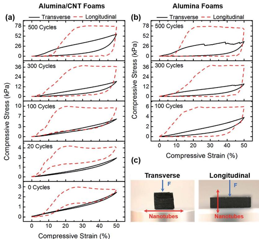
Fig. 3 Compressive stress–strain curves from first cycle of testing (a) alumina/CNT foams and (b) alumina nanotube foams in both transverse and longitudinal directions. Schematic provided in (c) to illustrate nanotube alignment relative to direction of compressive load.
